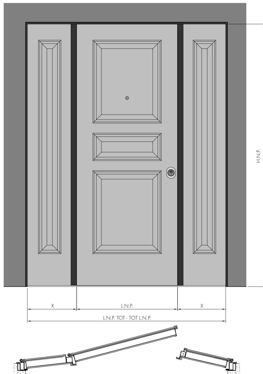
$$X \text{ (MISURA ANTINA)} = (\text{L.N.P. TOT.} - \text{L.N.P.})/2$$
