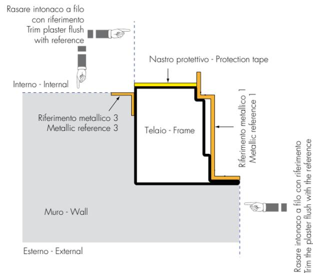
**MONTAGGIO COMPLANARE INTERNO CON CORNICE (90X12)**
